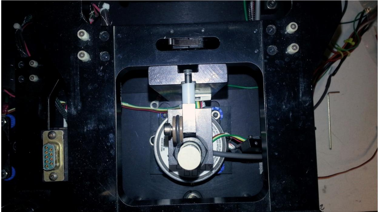
Output CAP sensor installed, top view
