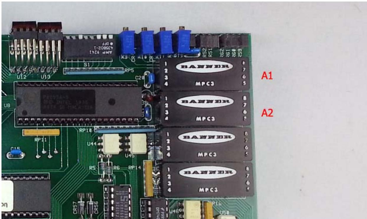
5. Install the Capacitive Sensor Board PN 5106-000012
