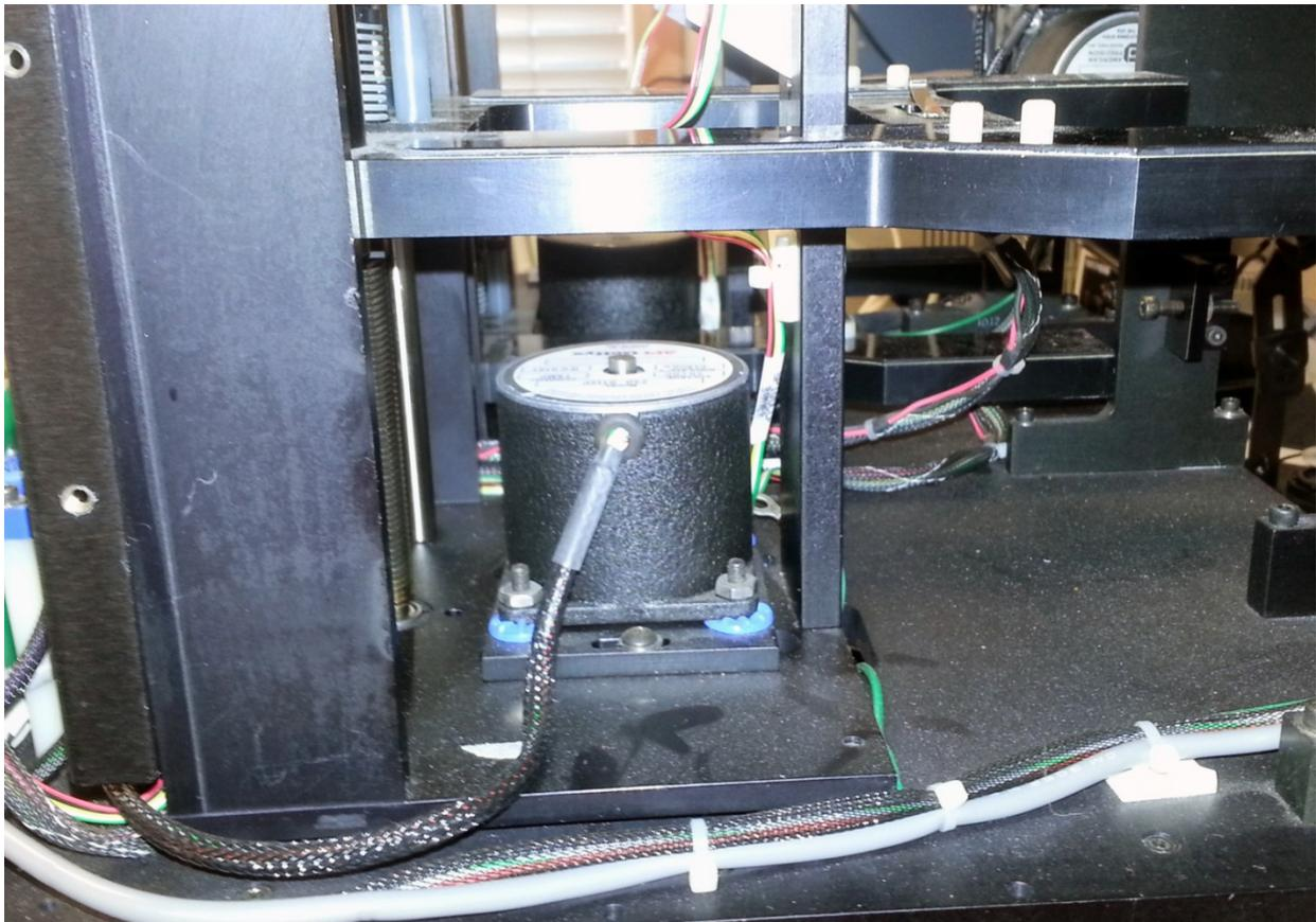
Modified Output Stepper Motor, with the shaft cut so it does not interfere with sensor.
