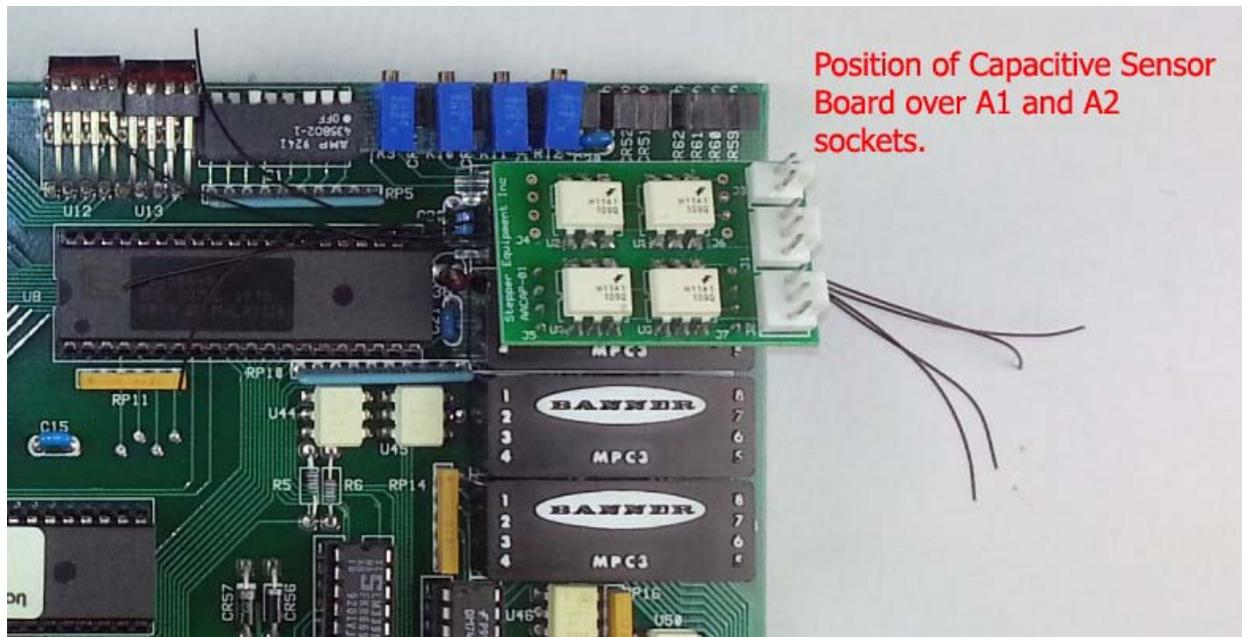
6. Flip the main board over so the back is exposed. Solder the 8 pins coming through the A2 holes to the corresponding pads. Cut off any excess pins.
