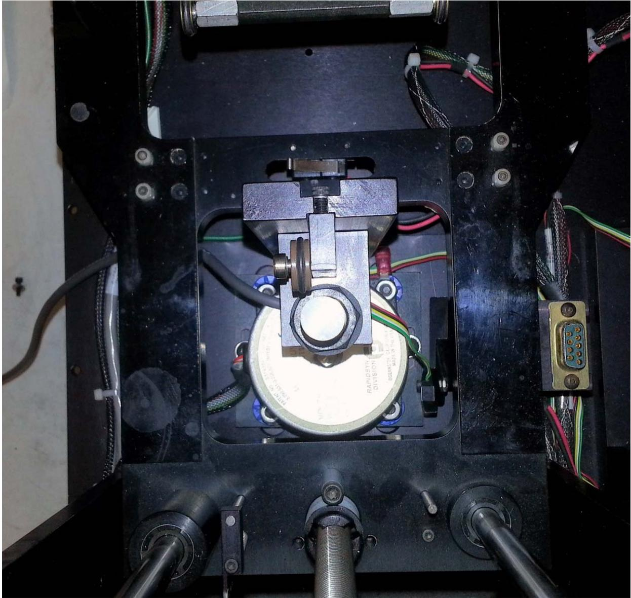
Top view of Input Cap sensor installed in bracket.
