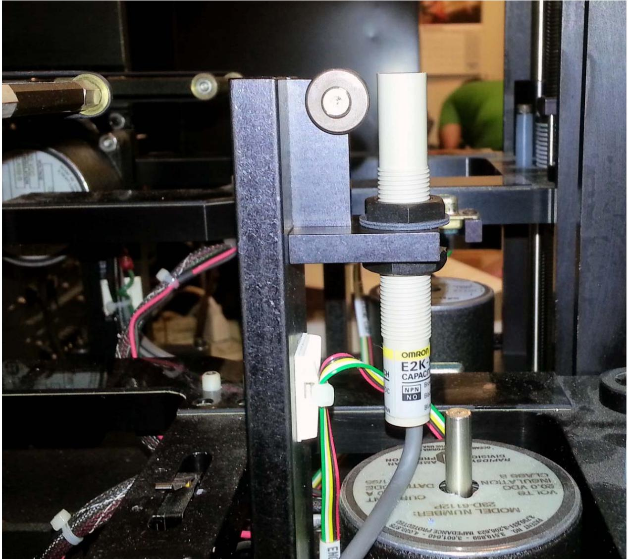
Side view of Input Cap sensor installed in bracket and mounted.
