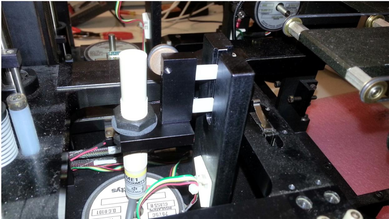
Side view of Output Cap Sensor installed, with spacers. This sensor sits farther back so the wafers go completely into the cassette.
