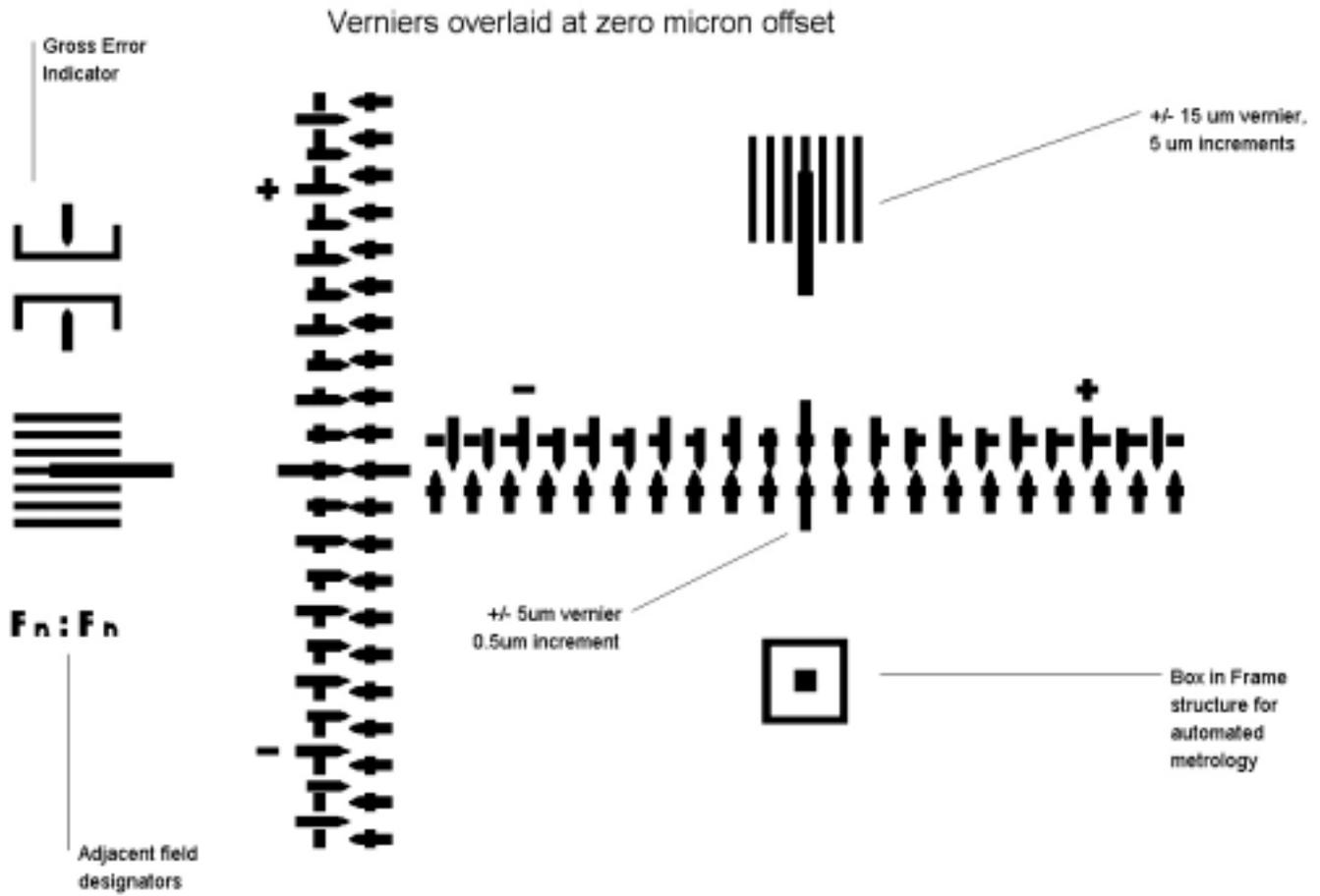
Figure 3 Verniers aligned with 0 offset
